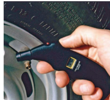
While doing that, check for wear and damage. Tyres must have a minimum of 1.6mm of tread over the central 75 per cent of the tread width for the whole circumference. However, trailer tyres often perish long before tread wears out, so look for the telltale
